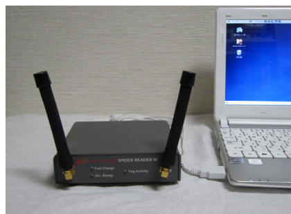
Figure 4. RFID reader and a notebook computer for data acquisition and processing.
