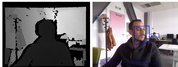
Fig. 1. The raw input depth from the tracker (left) and the head pose estimate superimposed on the input color image.
