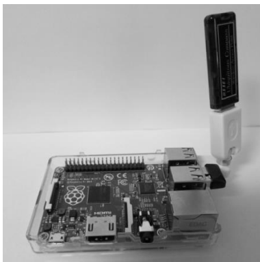
Figure 5. Small computer with an RFID reader inserted in its USB port.
