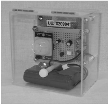
Figure 4. Front side of the IR motion sensor (an IR sensor module with a Fresnel lens and an active RFID tag at the back side).
