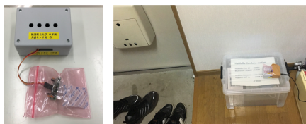
Figure 6. Motion sensor used near the entrance to detect a subject's arrival and departure.
