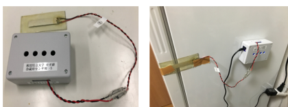
Figure 5. Refrigerator sensor. This is our originally developed sensor using a piezoelectric films bound with a urethane sheet.
