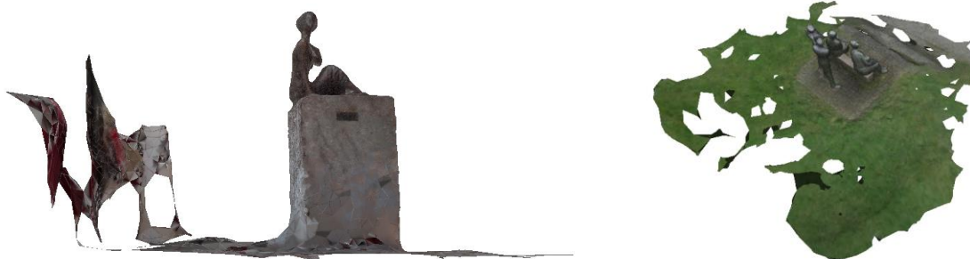
Figure 1. Two sculptures reconstructed from 186 pictures (left) and 176 pictures (right). Both are not oriented well for use in augmented reality applications and contain artifacts and unwanted surroundings.
