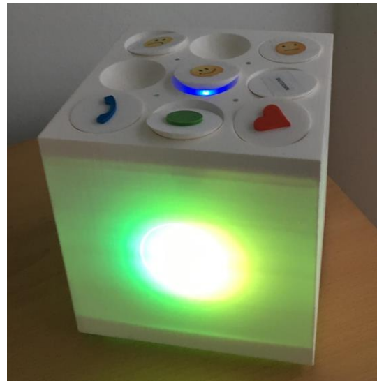
Figure 6. The RelaxedCare cube prototype that provides the overall wellbeing state of the assisted person via ambient lighting.
