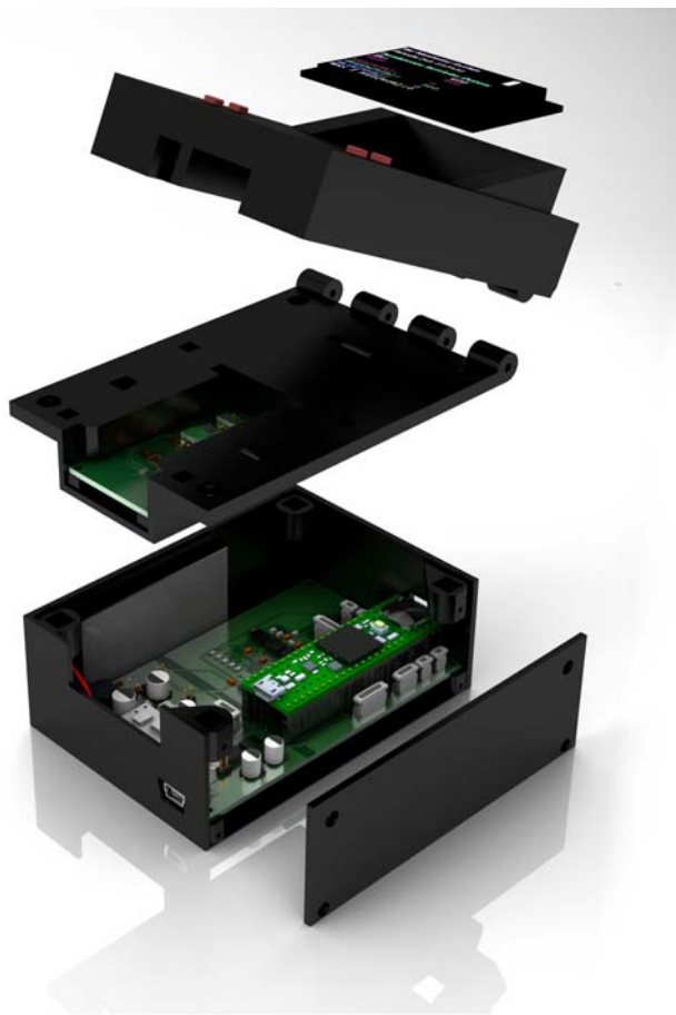
Figure 2. Design of the measurement device, useable as an about fist-sized, stand-alone, mobile monitoring and analysing system. Exploded view showing, top to bottom, the display and control elements, the measurement chamber and the electronic components, microcontroller-board, SD-card slot and USB port.
