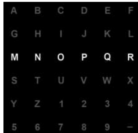
Figure 1. Common P300 speller matrix proposed by Farwell and Donchin. It consists of a 6 x 6 matrix of grey letters and numbers and black background.
