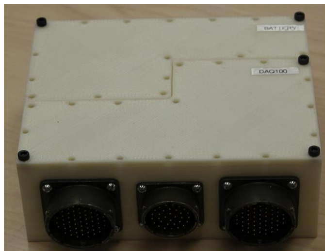
Figure 7. DLS System enclosure
