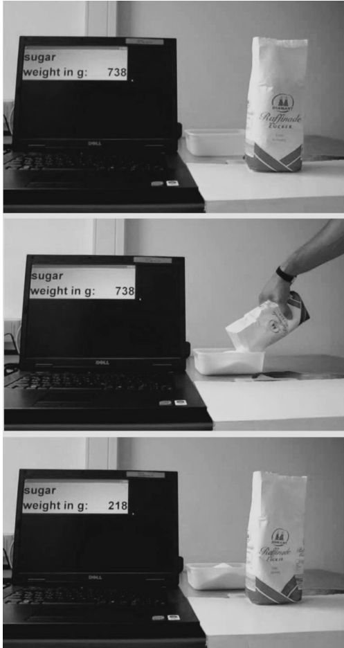
Figure 3. Three screenshots of an exemplary fill level measurement by using a scale and RFID (stucked on the shelf)
