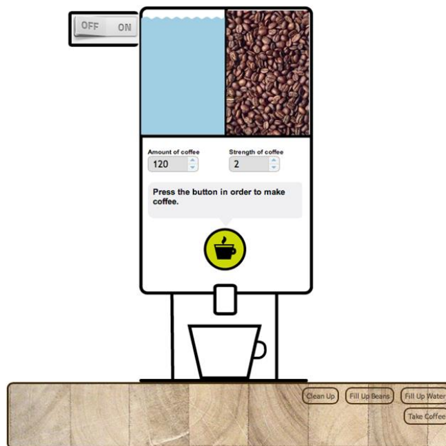
Figure 4. A Web client for a coffee machine. The upper-left button indicates that the coffee machine is switched on. The user can select the strength (1-3, i.e., weak to strong) and the size of the coffee cup (50ml to 150ml). The user receives notifications if either the water or the coffee reservoir is empty or the machine needs cleaning.
