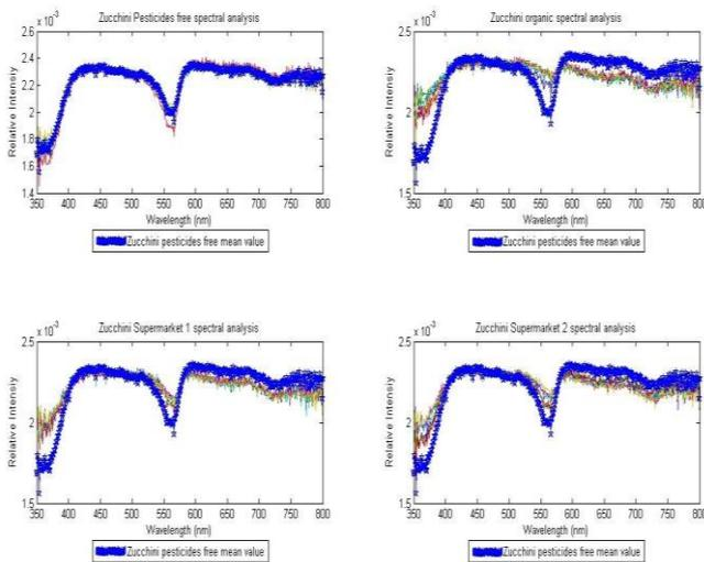
Figure 4. Zucchini spectral data comparison. The sample data are displayed by the colored thin lines and the mean value (only associated with the pesticides free spectrum) is depicted with the thick blue line.
