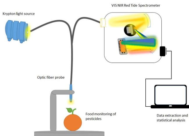
Figure 2. Test bench diagram used for Vis-NIR spectroscopy measurements in various vegetables
