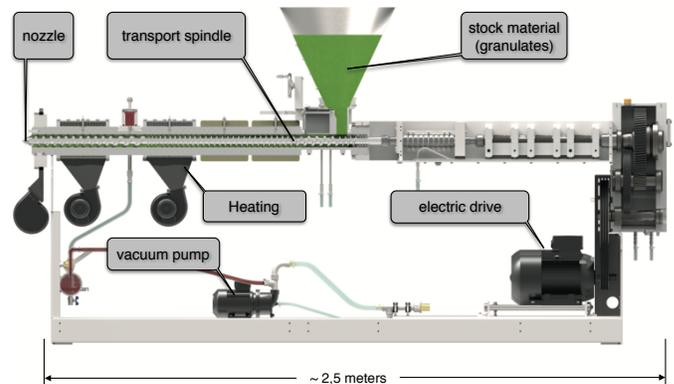
Figure 1. Working principle of an extruder
