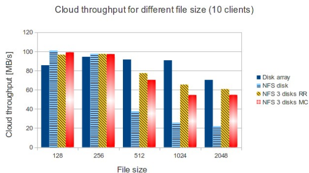
Figure 4: The Cloud throughput depending on a file size with 10 clients run in parallel.
