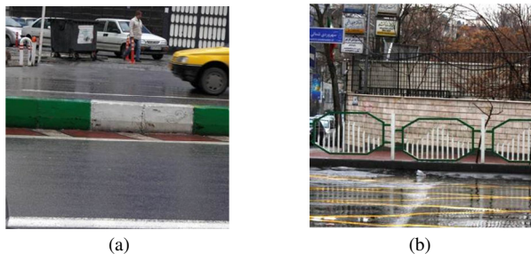
Figure 5. Examples of edges: (a) An impassable hard edge for a car, but passable for a pedestrian; (b) An impassable hard edge for both cars and pedestrians
