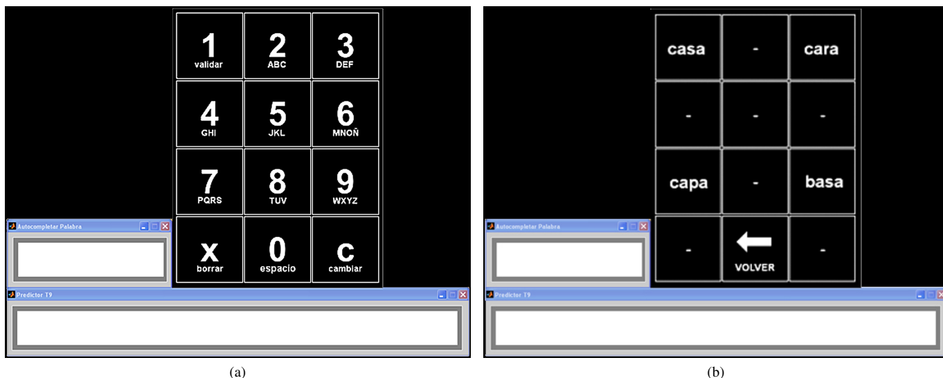
Figure 2. The two different interfaces of the SpellerT9. (a) The 4 x 3 virtual keyboard for typing. The text box below the keyboard showed the user’s message interpreted by the predictive text system, while the text box to the left displayed the outcome of the word predictor. (b) In case the textonym selected was not the word desired by the user, he/she could disambiguate the key selection by choosing among the four most frequently used textonyms. In the figure, the selected keys would have been 2272. See text for details.
