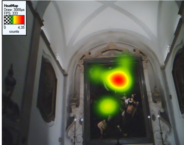
Figure 3. Heatmap by Tobii Studio software visualizes in real time the intensity in the observation of the picture (Fixation Count).
