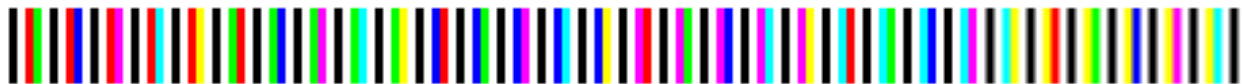
Figure 2. Structure Light Pattern containing 30 unique color edges. Total number of edges to be extracted from one 2D image is 153.
