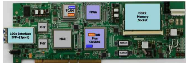
Figure 3. OCTEON CN5860 Network Processor based Deep Packet Processing Card
