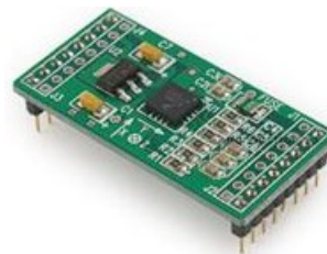
Figure 2. MMA7260Q accelerometer coupled in your circuit for ease of manipulation [14].
