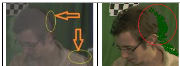
Figure 7: (a) Misalignment of the color image and depth map (b) part of the hair on the right of the hole is identified as a background.
