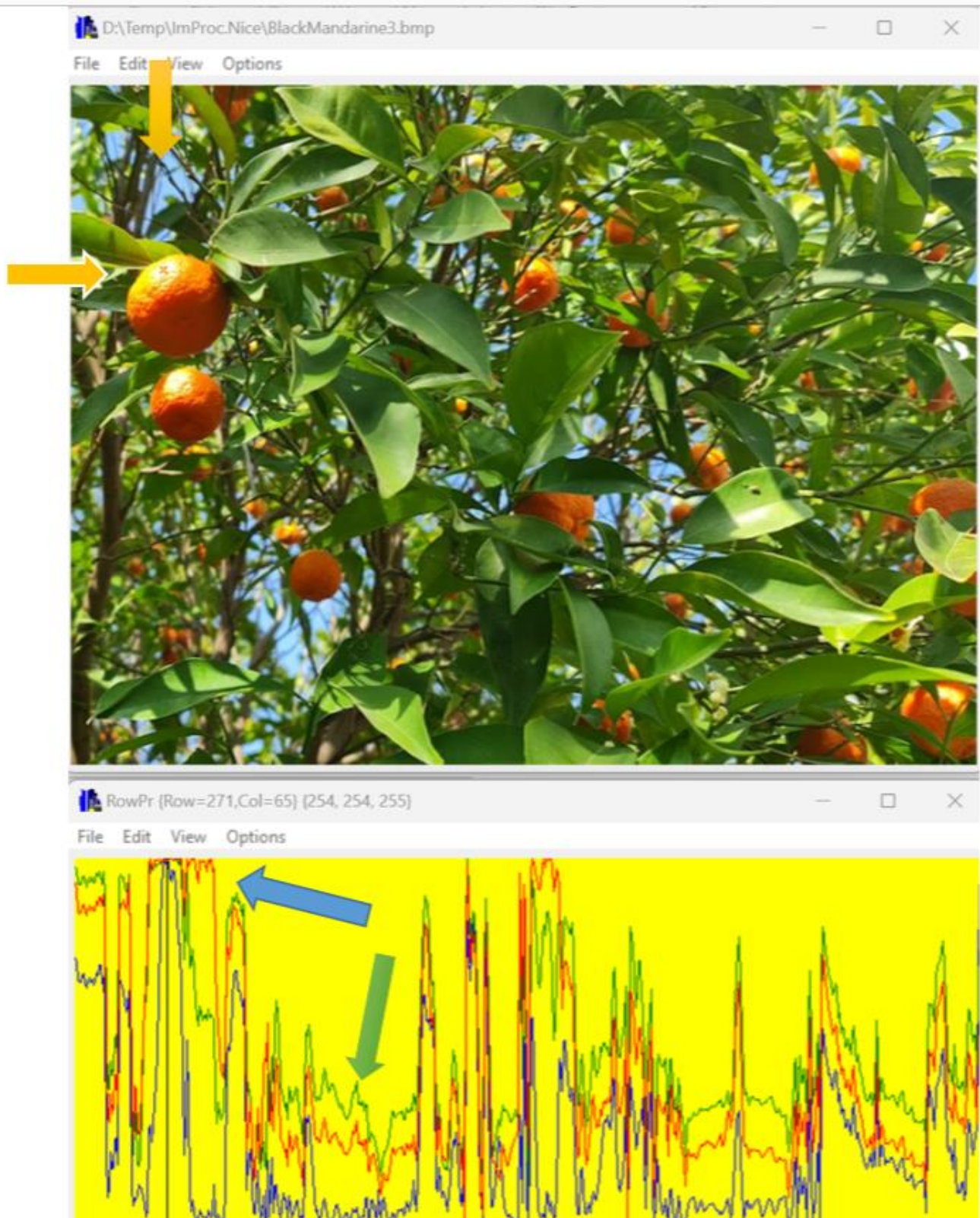
Figure 1. Real-life image of mandarines and profile of the row marked by a cross and by orange arrows. Blue arrow points to the overbleached region. Green arrow points to the unrealistically low blue values.
