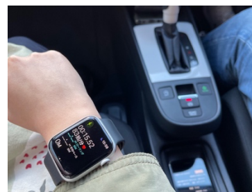
Figure 5. Measurement of passenger’s heart rate using Apple Watch
