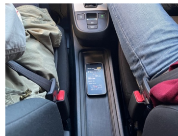
Figure 4. Measurement of vehicle speed and angular velocity using smartphone sensors
