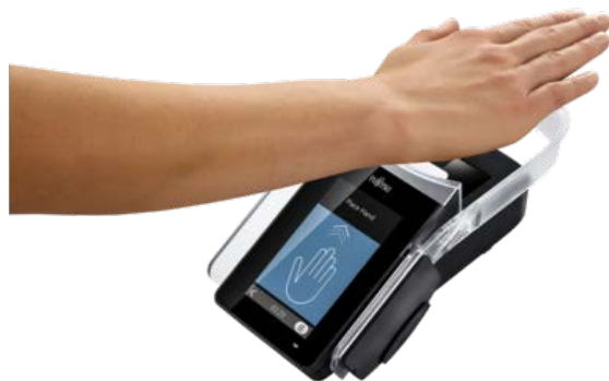
Figure 3. Example of a (palm) vein scanner: Fujitsu’s PalmSecure ID Match [14].
