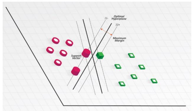
Figure 1. Optimal hyperplane within a two-dimensional space
