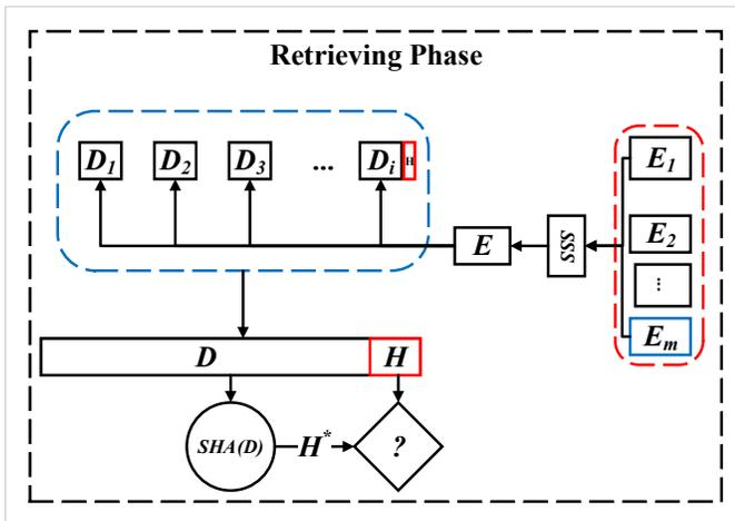
Figure 5. Schematic diagram of the Retrieving phase
