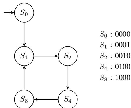
Figure 1. Stepper motor control specification TS
