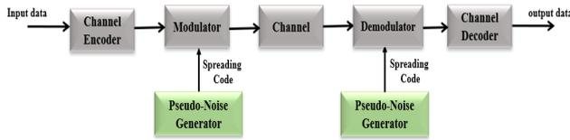
Figure 3. Model of Spread Spectrum Digital Communication System [6]
