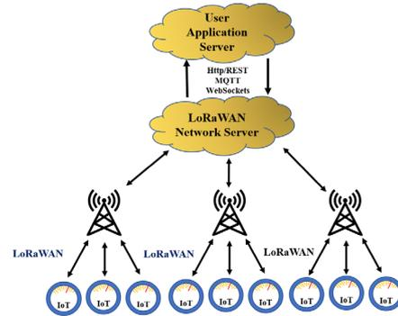
Figure 5. LoRaWAN Architecture [19]
