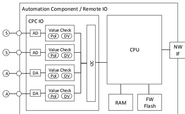
Figure 5. Automation Component with Integrated Physical World Firewall
