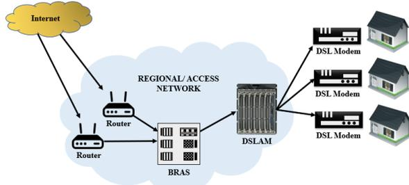
Figure 1. DSL Deployment and the Component [3]
