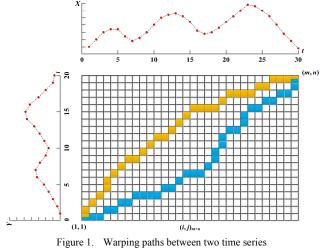
**Definition 3** Suppose time series  $X=(x_1,x_2,...,x_m)$ ,  $Y=(y_1, y_2,...,y_n)$ ,  $m \ge 1$ ,  $n \ge 1$ , then the DTW distance between X and Y is
