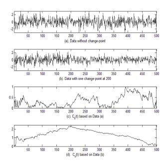
Figure 1. Top two panels: (a) data without any change in distribution; (b) data with one change in distribution at  $k^* = 200$ . Bottom two panels: plots of  $C_k(t)$  with t = 0.2 based on the data displayed respectively in (a) and (b).
