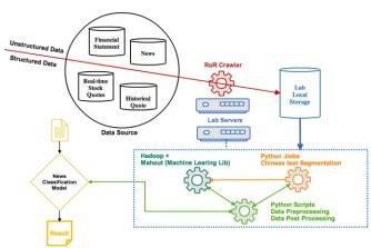
Figure 1. Workflow of the System.
