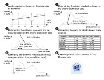
Figure 2: Q-AURA process in detail
