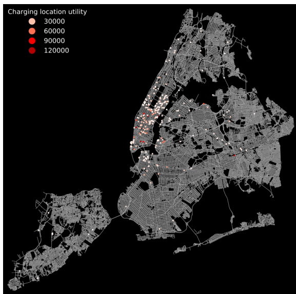
Figure. 10. Charging station utility map.
