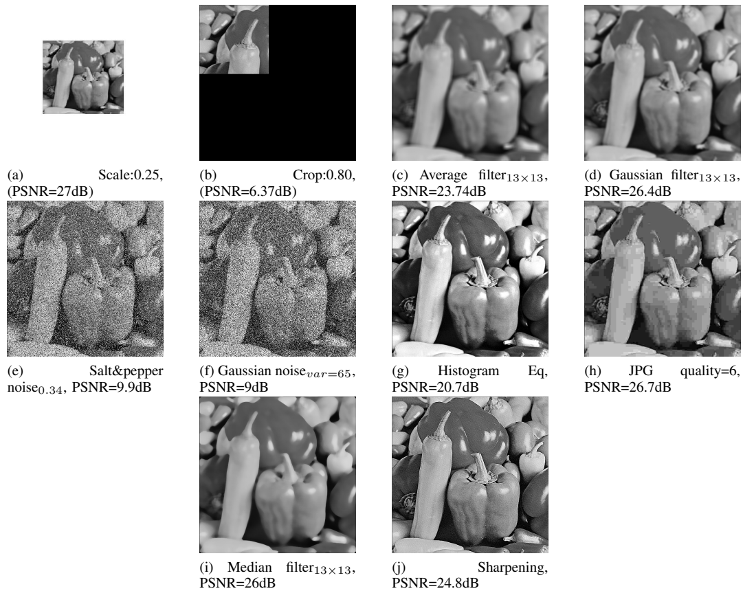
Figure 12: Some used images for evaluating the robustness of algorithm against various attacks
