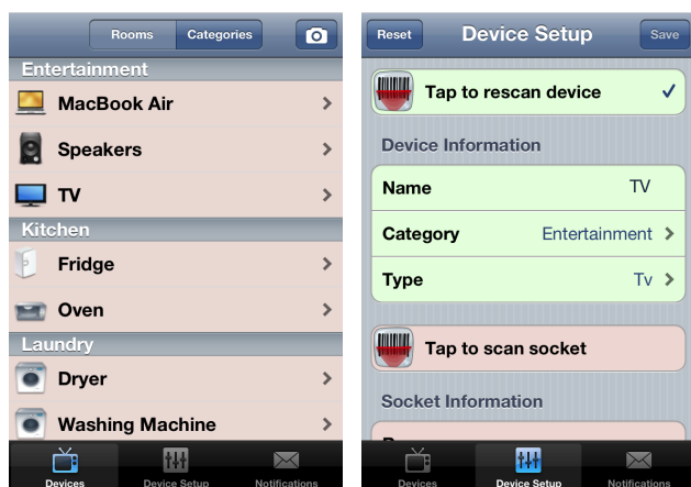
Figure 6: USEM devices (left) and new device set-up (right) screens of the mobile phone interface
