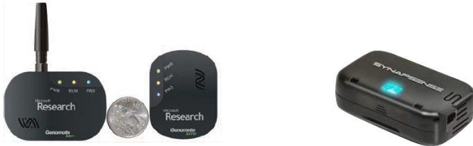
Figure 5. Sensor nodes for data centre monitoring. Left: Genomotes from Microsoft Research; Right: ThernaNode from SynapSense
