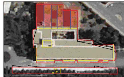
Figure 10. Common errors in the automatic vectorisation of the building edges and their corrections.
