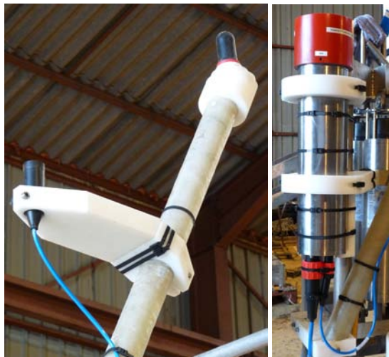
Figure 10: Views of the FFR hydrophone with the support and of the titanium laser container that contains the SEB.
