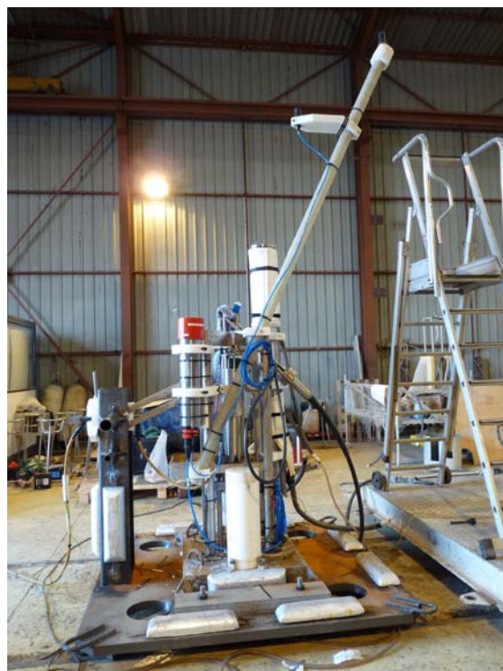
Figure 9: Picture of the anchor of the Instrumentation Line of ANTARES with the final integration of the transceiver.
