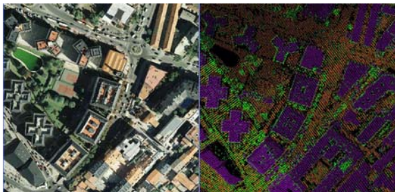
Figure 6. Classification of the buildings in purple (right) and validation with orthophotography (left).
