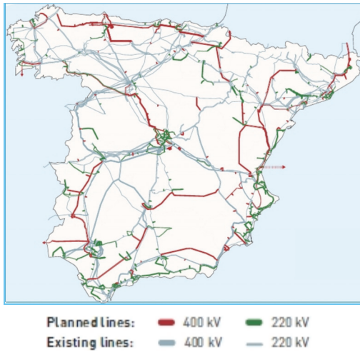
Figure 1. High voltage electrical energy distribution throughout the Spanish peninsular territory (adapted from [10]).
