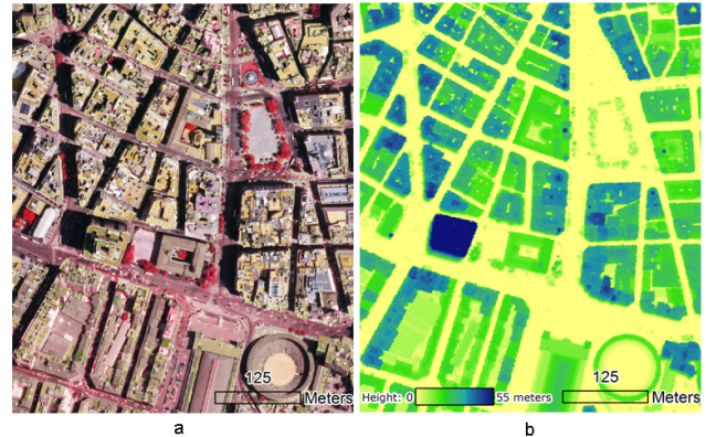
Figure 2. Detail of a high spatial resolution image in colour infrared composition (a), and digital surface model created with the LiDAR data (b), depicting a zone in the urban centre of Valencia.
