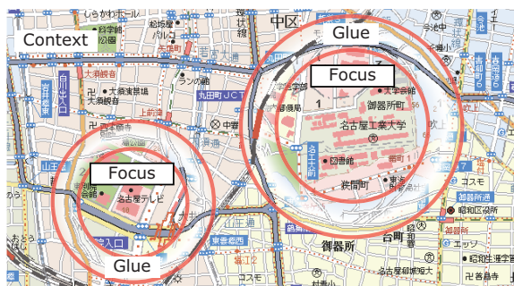
Figure 8. “Focus+Glue+Context” fisheye view maps in Emma. Users can adjust the size, position, and scale of the Focus by mouse-dragging.
