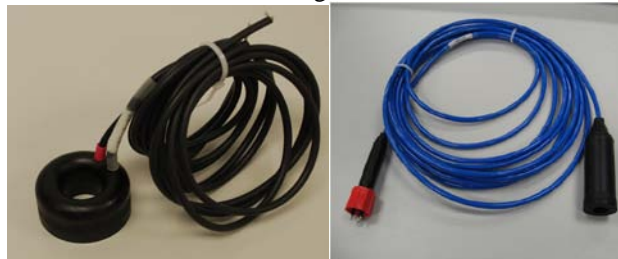
Figure 1: View of the Free Flooded Ring hydrophone (without and with over-molding).
