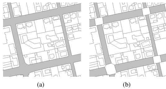
Fig. 3. (a) Original NGB street polygons and (b) enhanced by crossroads area polygons.
