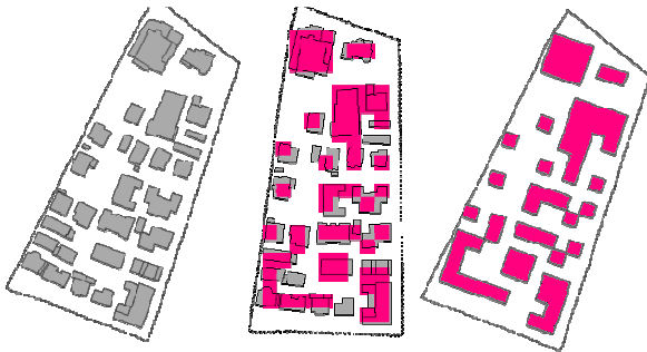
Figure 5. The Generalization Process of Buildings in a Quarter: Original Buildings (left); Rotated Quarter and the Generalized 10 meter Rasterized Buildings in red (middle); Final Result (right).
