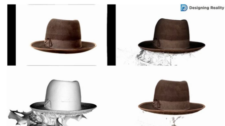
Figure 9. A Designing Reality model of the hat: Photograph, Point cloud, mesh and mesh with texture.
