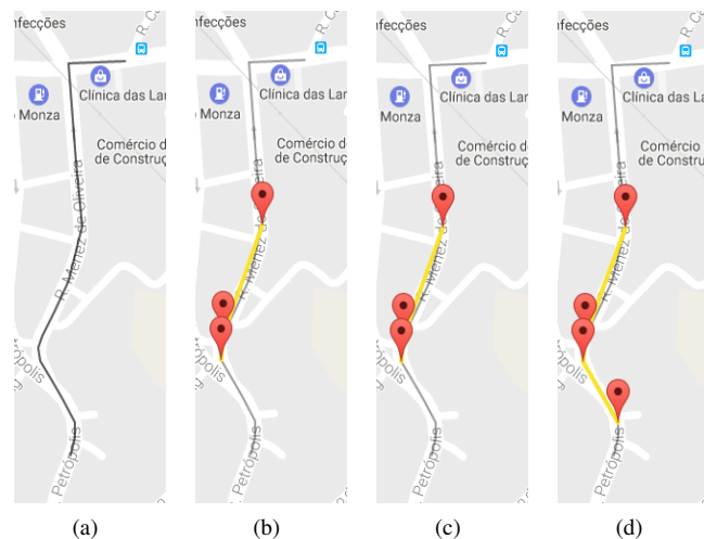
Figure 8. Experiment with identical trajectories - (a) original trajectory (b) ( \epsilon = 0,00015 ) (c) ( \epsilon = 0,00020 ) (d) ( \epsilon = 0,00030 ).
