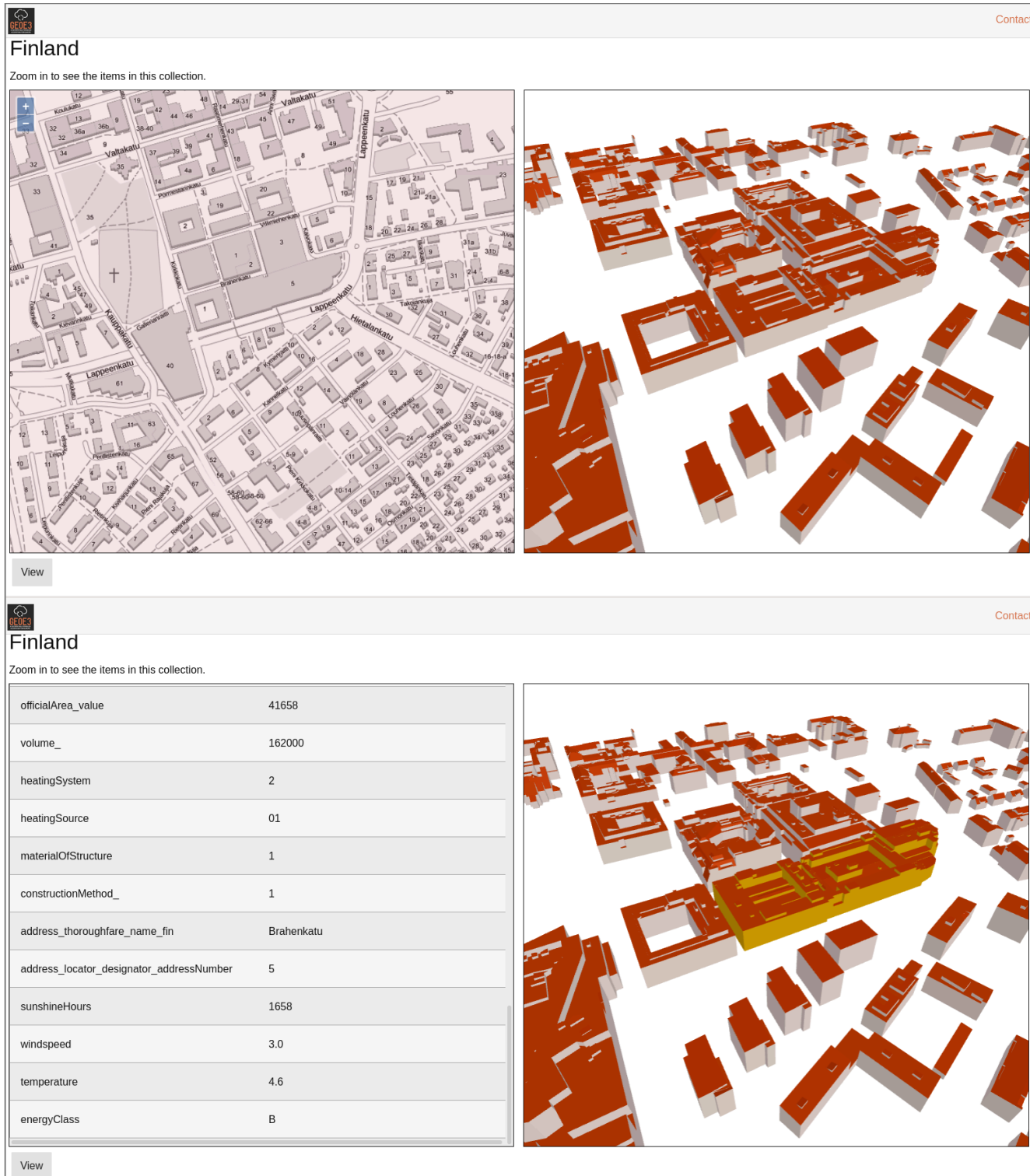
Figure 3. City block-level view of the 3D buildings, requested by a BBOX query from the OGC API Features service of the GeoE3 platform (top). Attribute display of the selected building with technical, climate and energy related attributes shown (bottom).
