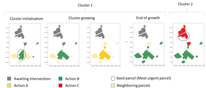
Figure 1. The cluster growing procedure applied on 12 polygon-based parcels, with 3 possible actions. Resulting in 2 homogenous clusters.
