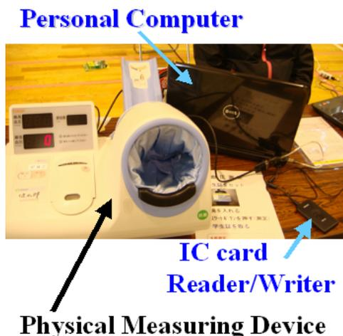
Fig. 5. Photo of a Blood Pressure Monitoring Device as physical measuring device, IC card Reader/Writer and Personal Computer in the routine physical examination.
