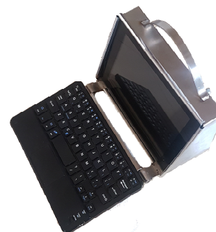
Figure 3. Portable central unit based on Raspberry Pi.
