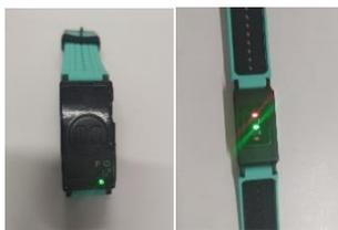
Figure 1. Device used (MAXREFDES103).
