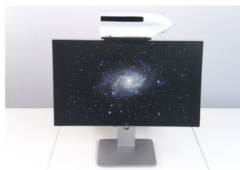
Figure 1. A ergoscan device mounted on top of a monitor.
