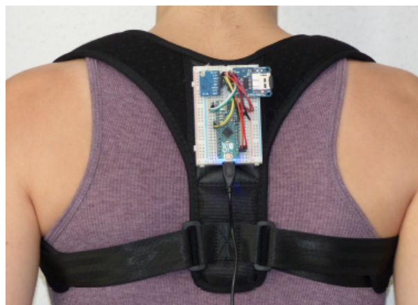
Figure 1. Wearable sensor platform fixed at a test subject's upper body.
