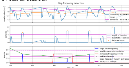
Figure 4. User low steps frequency detection . (a) Potential step detection, (b) step validation, (c) low steps frequency detection
