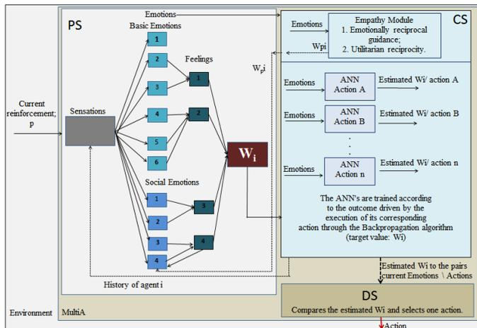
Figure 1. The general scheme of the MultiA Architecture.
