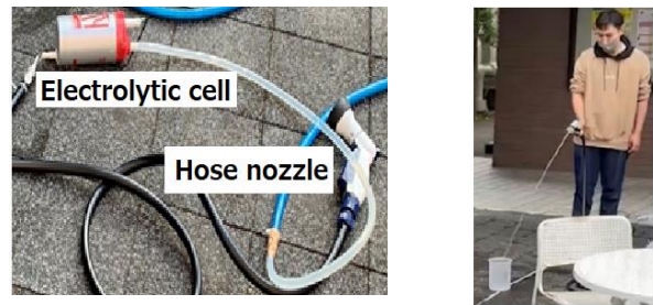
Figure 4. Prototype of the flowing water device for producing ozone water (left), and procedure for measuring the ozone concentration at various distances from the hose nozzle (right).
