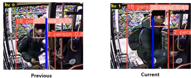
Figure 12. Before and after passengers cross the baseline.
