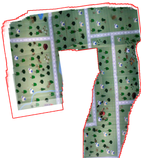
Fig. 8. Comparison between new and old scaling method. Shown are the registered images using the new scaling method. The underlying contour marks the extent of the registered images, if the old scaling method would have been used.
