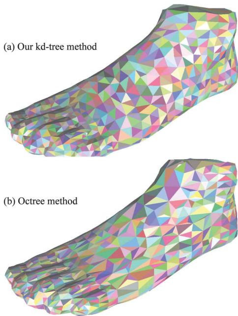
Figure 5. Examples of simplified meshes with a mesh Foot. In (a), the mesh is simplified to 1,104 vertices using our kd-tree method whereas in (b), the mesh is simplified to 1,206 vertices using the octree method.
