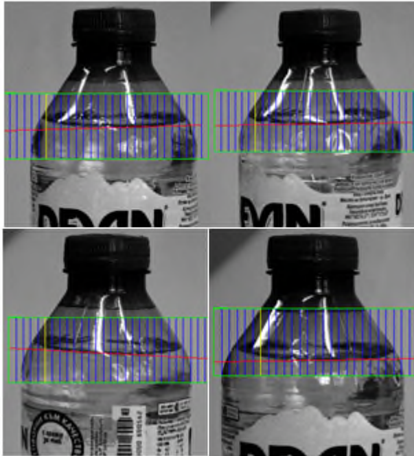
Figure 10. Line fitting for bottled mineral water - edge strength 32, kernel size 9, projection width 9 and interline gap 77 pixels
