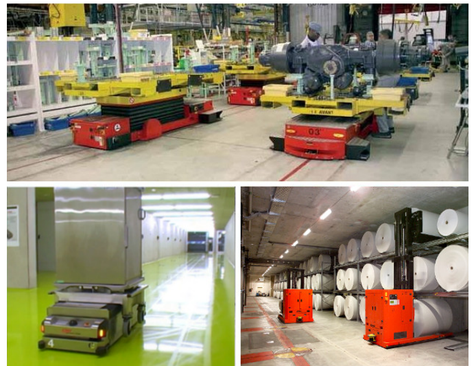
Figure 1. DS-Automation's AGVs in action on an automotive assembly line, in a hospital and a paper factory.
