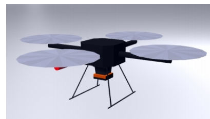
Figure 2. The Hector quadrotor rendered within the Gazebo simulator. Image taken from [12].
