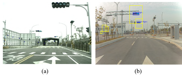
Figure 4. (a) The projection of traffic lights' center points. (b) ROI generation according to the projection from the map.
