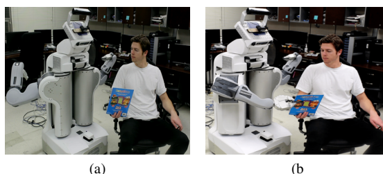
Figure 13. (a) Initial Pose of the Right Gripper and a Sticker-book. (b) Side Grasp of the Sticker-book.
