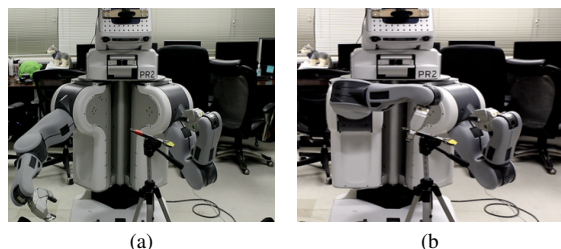
Figure 9. (a) Initial Pose of the Right Gripper and a Wrench. (b) Side Grasp of the Wrench Using the Right Gripper.
