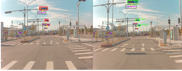
Figure 5. Data association between detection results and projection (gray virtual box).
