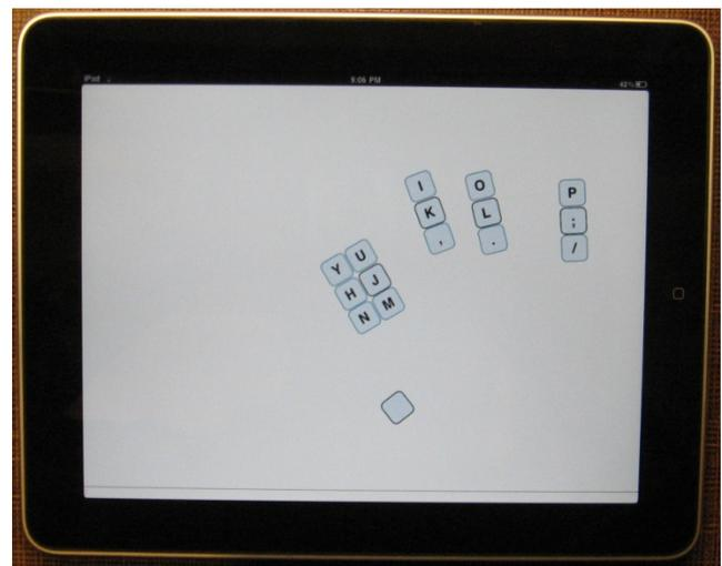
Figure 4 – The left photo shows the second LiquidKeyboard prototype on an Apple iPad. The right picture shows how the keyboard adapts to the shape of the user's hand.
