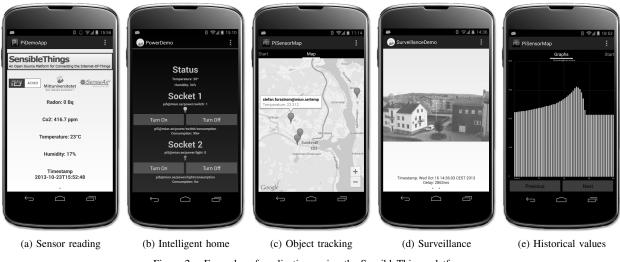
Figure 2. Examples of applications using the SensibleThings platform.
