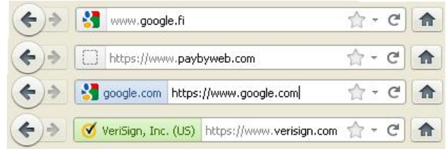
Figure 1. Security indicators in address bar of Mozilla Firefox 8 (from top to bottom: unsecured HTTP, ignored certificate error, regular certificate, extended validation certificate)
