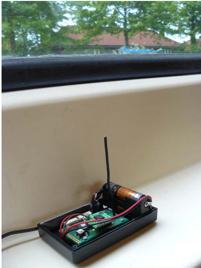
(a) Wireless sensor node
