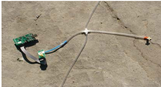
Figure 2. Mp3v5050gp Pressure Sensor Connected to TelosB Mote
