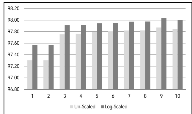
Figure 3: Average classification ratio values from the Cross-Validation, Logarithmic scaling versus unscaled feature space, K = [1,10]
