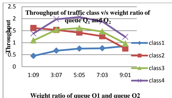
Figure 4: Variation of throughput for four classes of traffic v/s weight ratio for improved hybrid scheduler.
