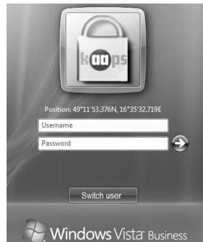
Fig. 8. Microsoft Windows Vista logon screens with integrated support of Multifactor Authentication Device (MAD connected-obtained position information, dialog used for user login)
