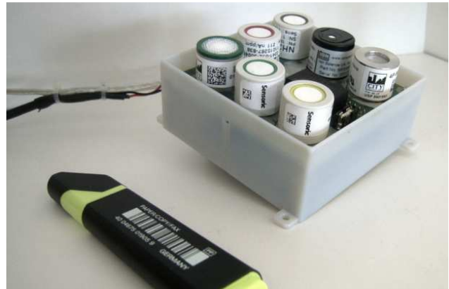
Figure 5. Gas sensor to detect inflammable gases, Ammonia, Nitrogen Dioxide, Sulphur Dioxide, Carbon Monoxide and Chlorine
